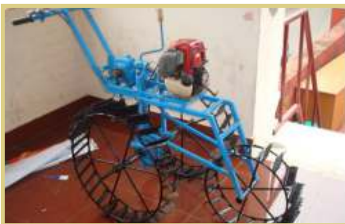
Photo 8.19 Three-row motorized weeder (TNAU)
