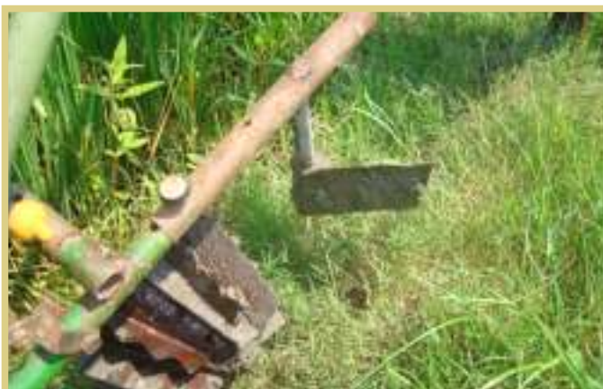
Photo 8.21 Small ridger attached to conoweeder
