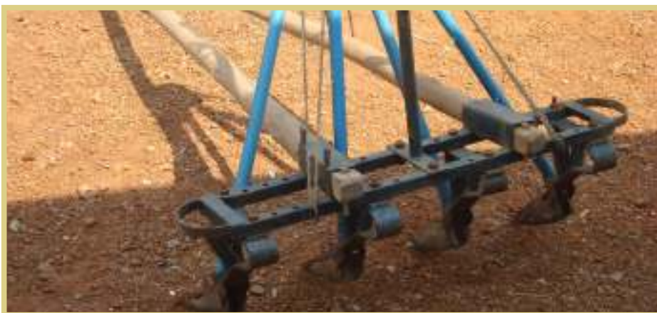
Photo 3.6 Four-row seed drill for rainfed SRI
